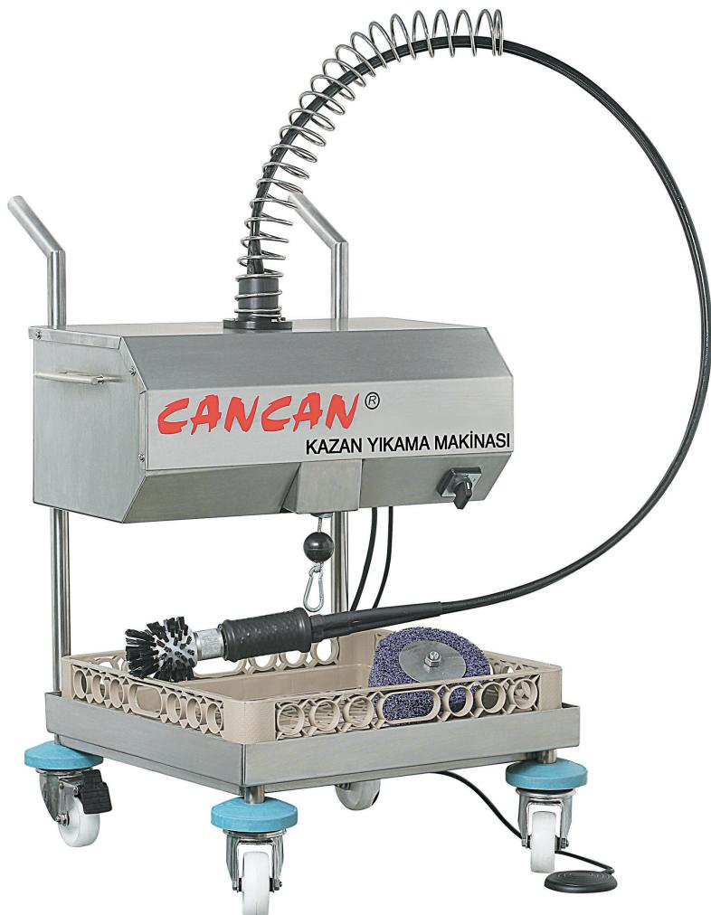
The pot washing machine is designed to clean the dirt and grease sticking to pots, pans and boilers in a short time, without requiring extra power in industrial kitchens with the help of the rotating brush or the polishing brush. This system can be used by mounted on washing sinks or can be used as a mobile cleaning brush everywhere in the kitchen with a trolley (optional) that can move in the kitchen. While it is used immobile, the body of the machine should be mounted at the height of 1,15 m.
